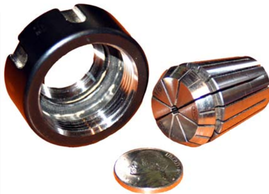
Typical Spindle collet and nut
