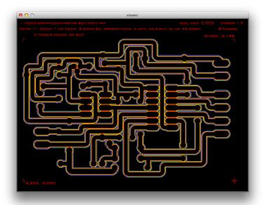
Figure 1.1: Preview showing color-coded multiple passes.
