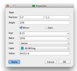
**Figure 3.11:** The object info for the mirrored text on the Milling layer. Note that the Mirror checkbox is on. This indicates to pcb-gcode that the text should be engraved on the bottom side of the board.
