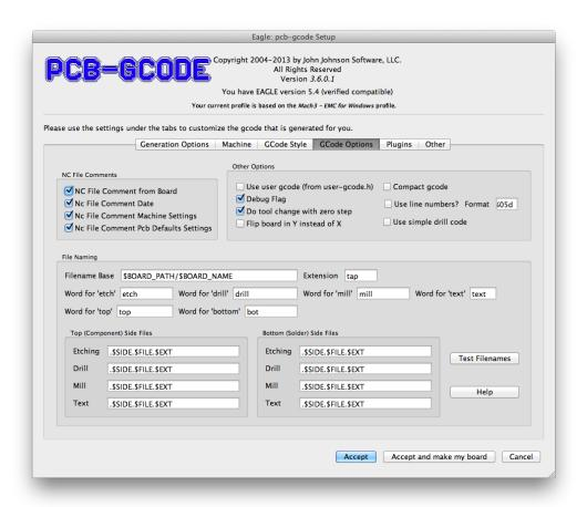
**Figure 2.7:** *Options for generating g-code files.*
