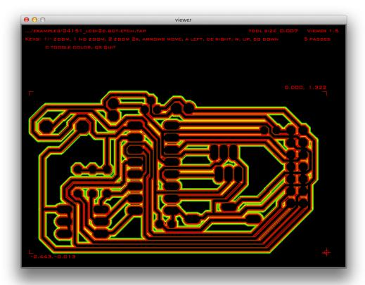
**Figure 3.7:** The previewer showing a multi-pass file for the bottom side of an example PCB included with pcb-gcode.
