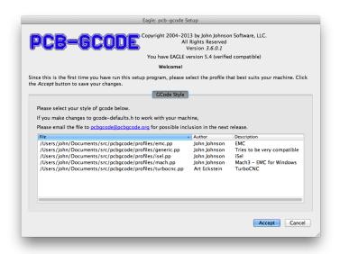
**Figure 2.3:** *Select the style g-code pcb-gcode should produce.*
