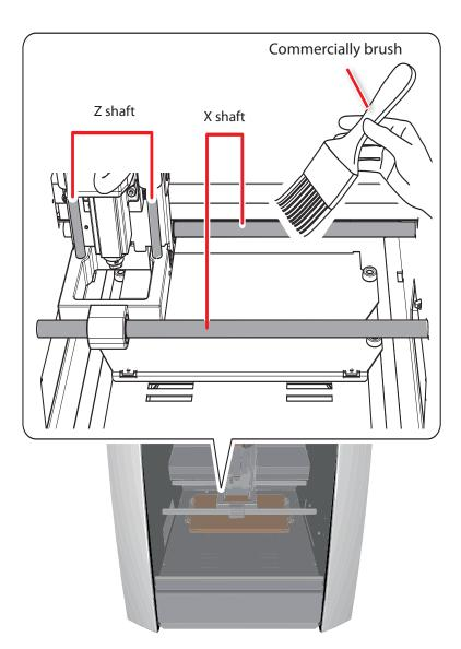
**5.** Brush the cutting waste down into the dust tray from the positions indicated on the figure below.
