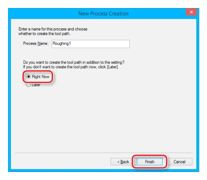
The tool path is created. And the process which is created is displayed.
