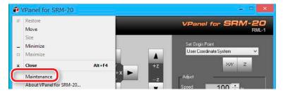
2. Check the total spindle motor rotation time.
