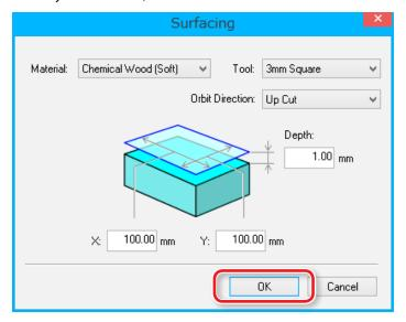
3. Make sure that the desired tool and origin position are correctly set up and then click Start Surfacing.
