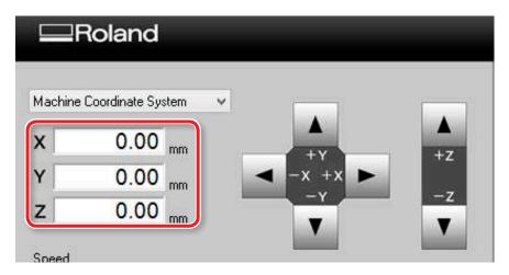
**4.** Select[User Coordinate System], check that XYZ is "0.00 mm." If "0.00 mm" does not appear for X, Y and Z, click [X/Y], then [Z] under set origin point.
