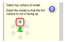
Changing the top surface changes the X, Y, and Z dimension values as well. A message appears if the size exceeds the movable range of the machine. Follow the prompts and take action accordingly.
