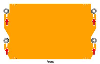
**6.** Tighten the screws firmly and return the front guard to the original position.
