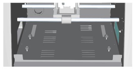
5. Fit the new table into the screw notches.
