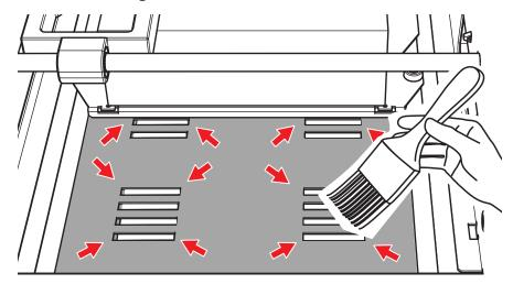
**6.** Remove the cutting waste that has collected in the dust tray.
