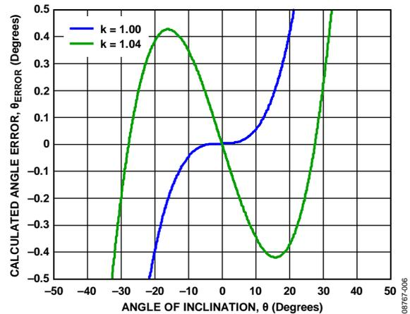
Figure 6. Calculated Angle Error for Different Scaling Factors
