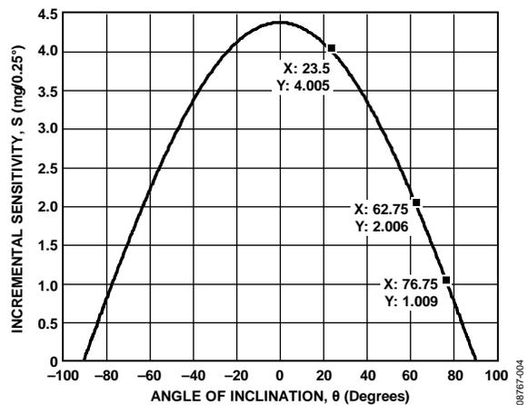
Figure 4. Incremental Inclination Sensitivity for 0.25° Steps
