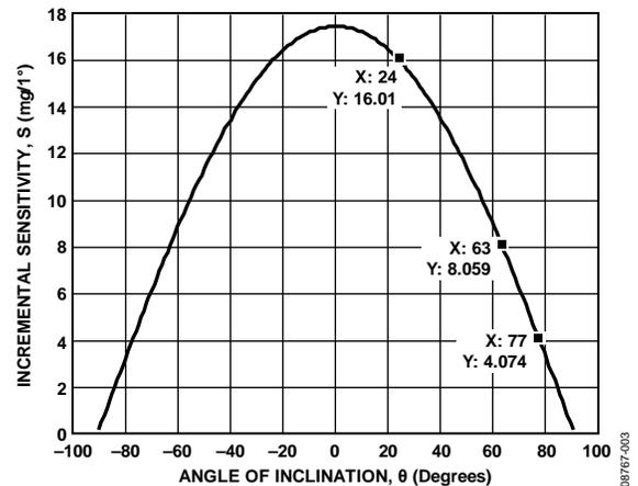
Figure 3. Incremental Inclination Sensitivity for 1° Steps
