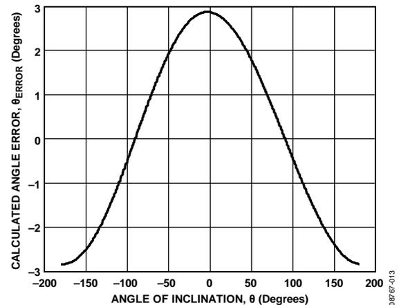
Figure 13. Calculated Angle Error Due to Accelerometer Offset
