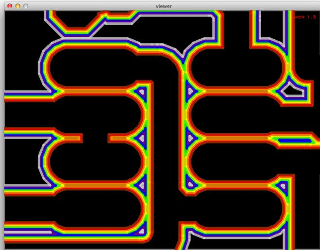
**Figure 1.2:** *Preview showing a zoomed version of the color-coded multiple passes. Brown is the first pass, red the second, orange the third, etc.*
