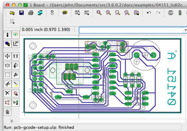
**Figure 3.8:** The sample board `docs/examples/04151_lcdi2c.brd` with wires and mirrored text on the Milling layer.
