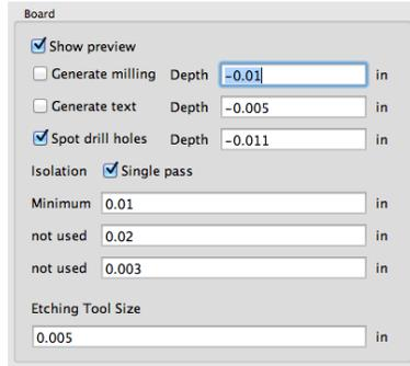
Figure 3.3: Pcb-gcode settings for the DRC example.
