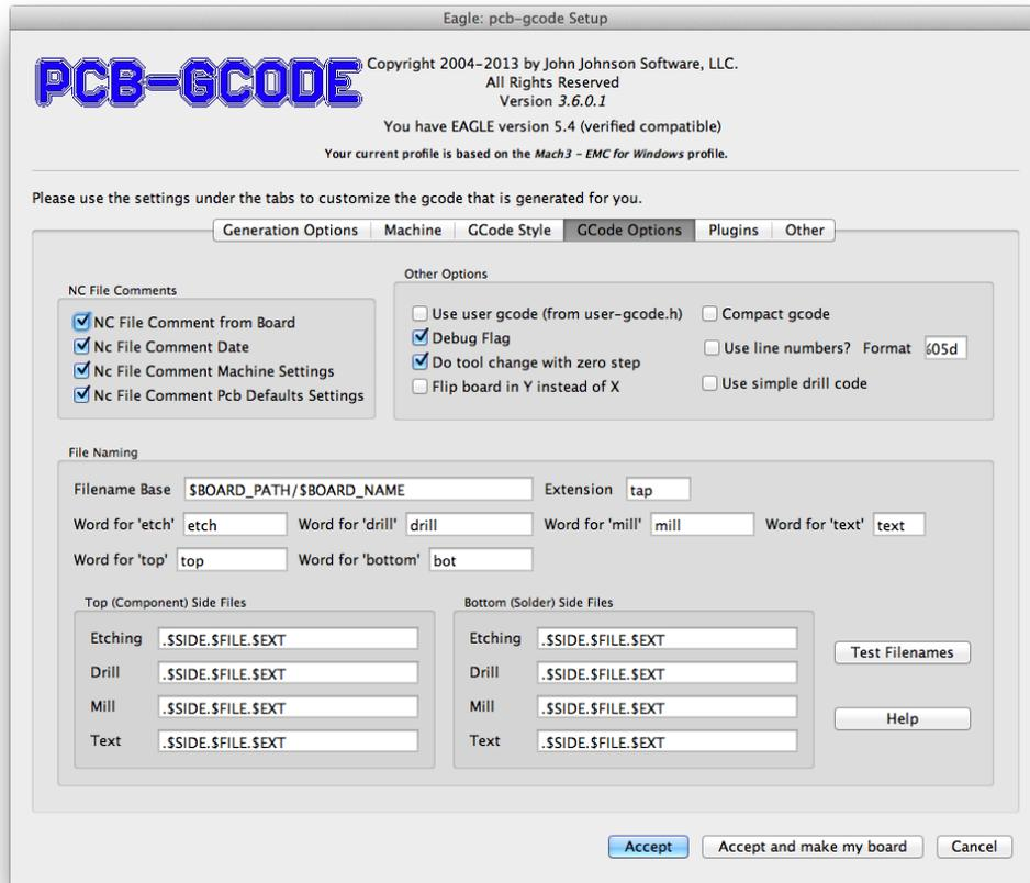
Figure 2.7: Options for generating g-code files.
