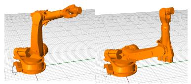
the same effector position in the elbow-up and elbow-down modes
