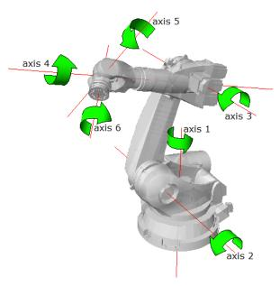
These 6 axes give the end effector (the part where the tool is attached - eg a gripper or drill) the full 6 degrees of freedom for location and orientation in space.
